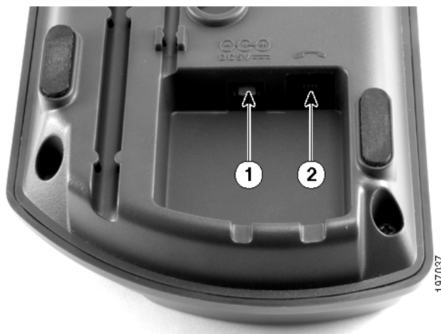
Figure 1 Cisco SPA 301 Phone Power and Handset Connections
