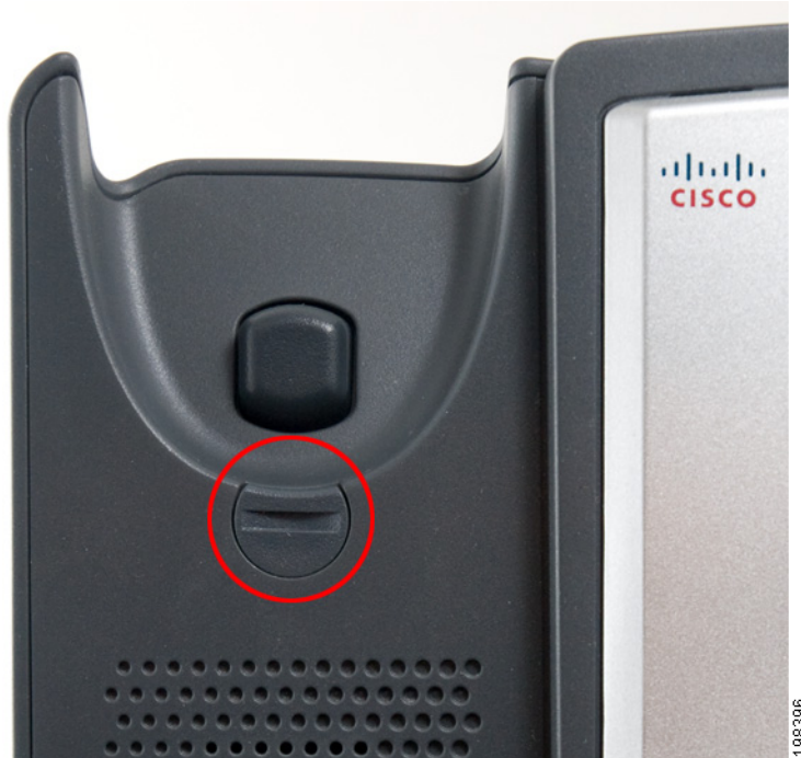
Figure 5 Handset Retention Tab (Default Position)
